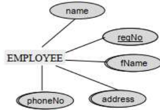
Figure No. 5.1: An Entity Type, its defining attributes and Super Key (underlined)
