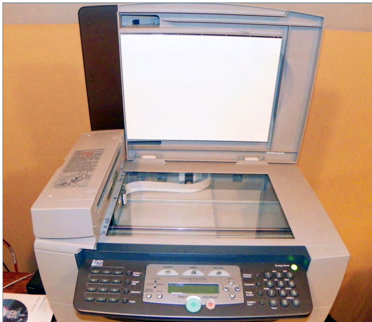
FIGURE 3.45 A flatbed scanner
