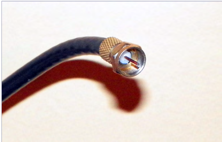
FIGURE 3.43 A CATV F connector and coaxial cable
