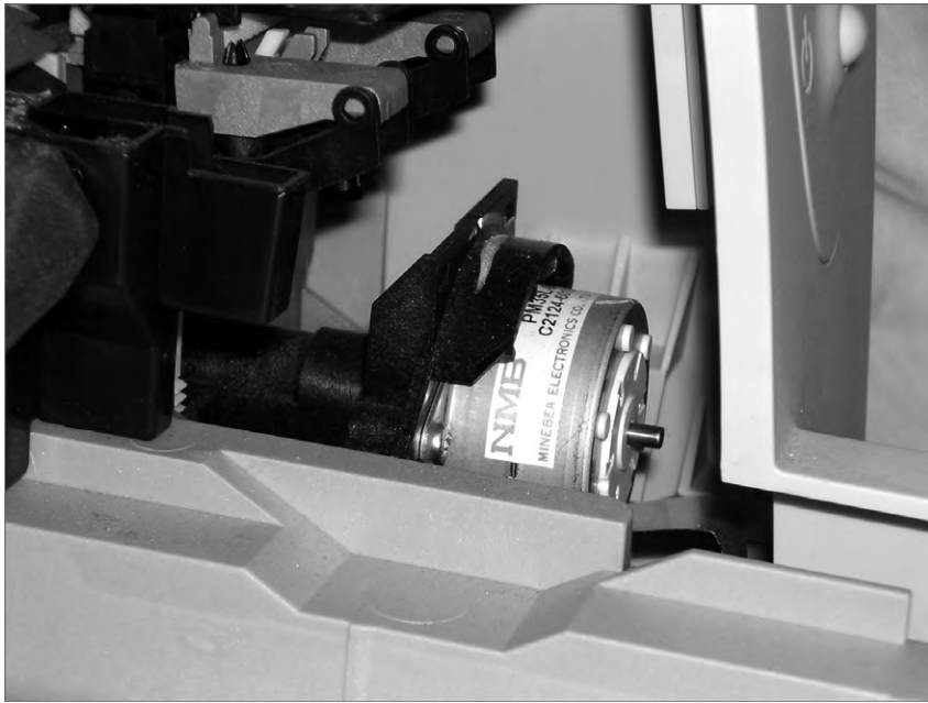
FIGURE 10.4 A carriage stepper motor
