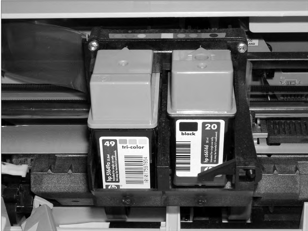
FIGURE 10.3 A print head carriage (holding two ink cartridges) in a bubble-jet printer
