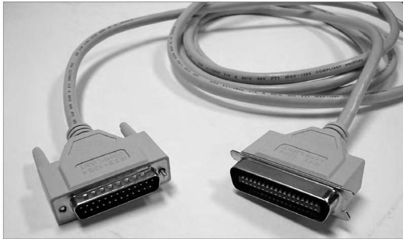
FIGURE 3.22 A typical parallel cable
