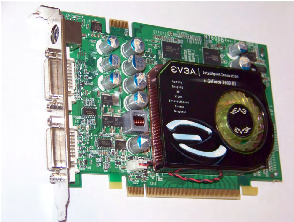
FIGURE 3.1 A video expansion card
