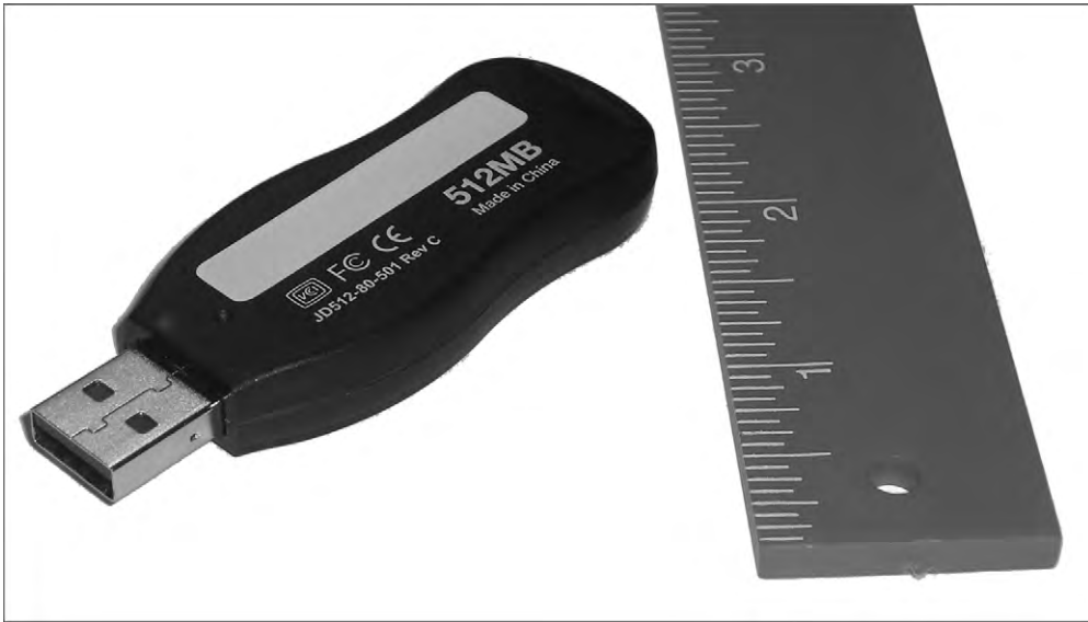
FIGURE 2.20 A USB flash drive
