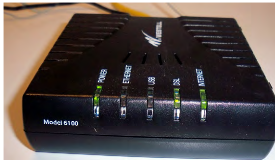
FIGURE 8.3 A DSL modem
