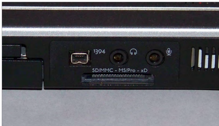
FIGURE 2.19 Memory-card slots in a laptop
