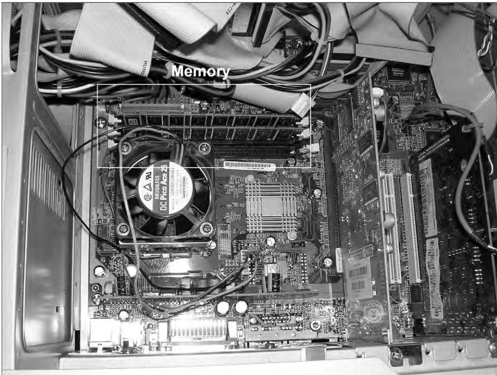
FIGURE 1.19 Location of memory within a system
