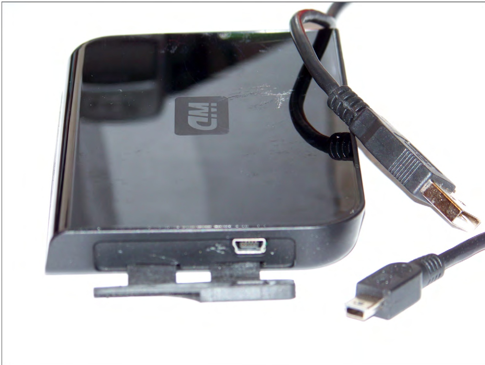
FIGURE 2.21 A self-contained external hard disk drive
