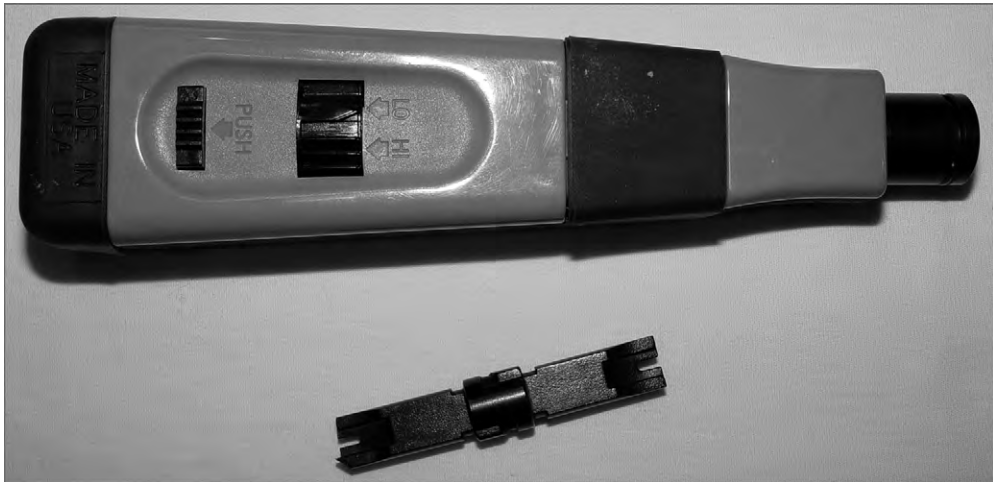
FIGURE 6.28 A punch-down tool
