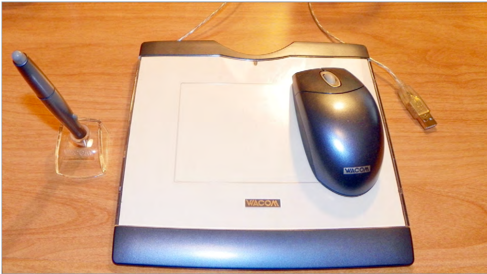
FIGURE 3.48 A digitizing tablet
