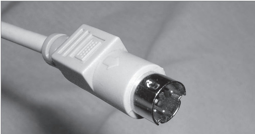
FIGURE 3.34 A PS/2 keyboard cable
