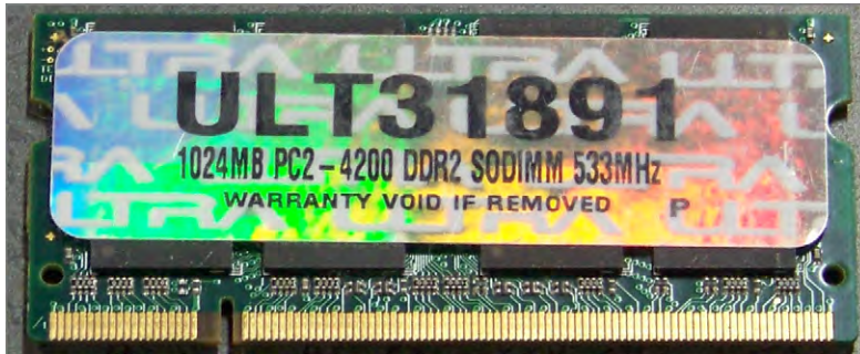
FIGURE 1.25 200-pin DDR2 SODIMM
