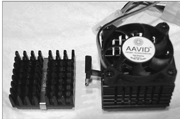
FIGURE 1.9 Two heat sinks, one with a fan
