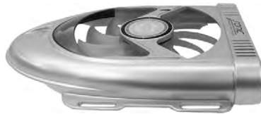
FIGURE 1.28 An active hard disk cooler
