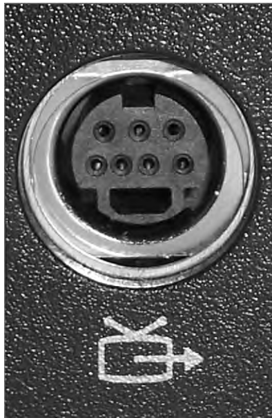
FIGURE 3.40 A 7-pin S-video port
