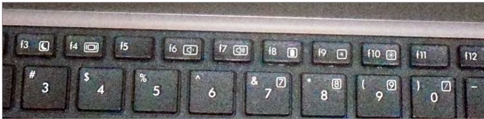
FIGURE 20.1 Video adjustment keys F4 (LCD toggle), F9 (dim), and F10 (brighten)
