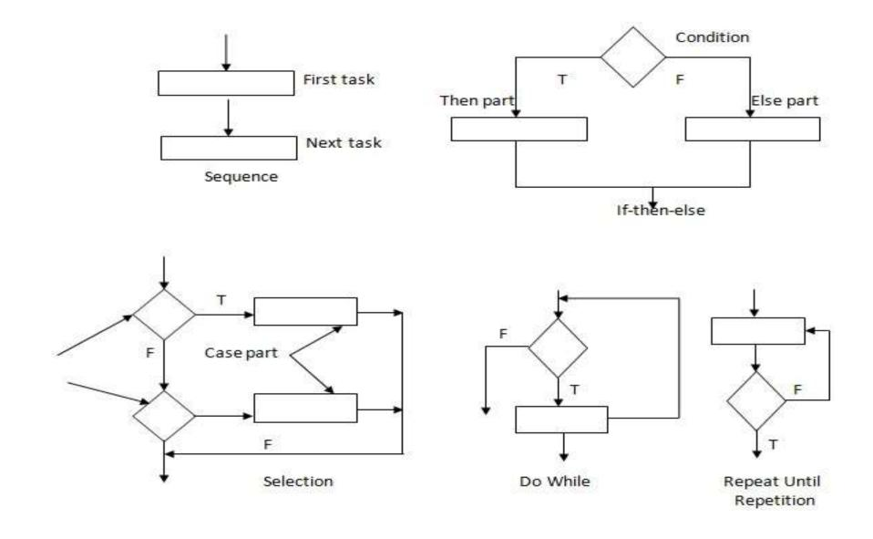
It show various flowchart constructs. Sequence is represented as two processing boxes connected by a line (arrow) of control.
