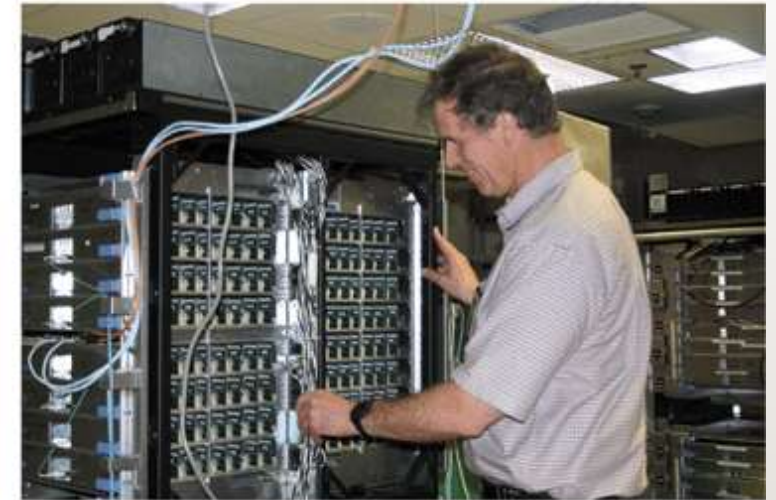
BLUE GENE/L CIRCUIT BOARDS Each rack holds several circuit boards; each circuit board contains four processors.
