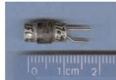
Figure 1.6 A transistor, replacing the vacuum tube Courtesy of Dr. Andrew Wylie
